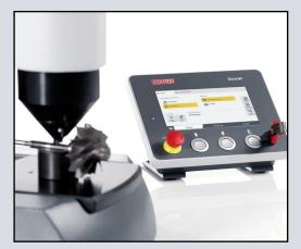
Hardness is a measure of the resistance to localized plastic deformation induced by either mechanical indentation. Hardness test is done by Rockwell, Vickers and Brinell methods.
