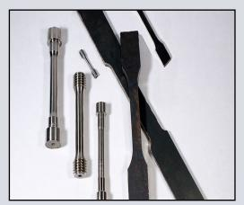
Tensile test is performed at different temperature to calculate the mechanical properties of rolled products such as yield strength, tensile strength, elongation and reduction area.
