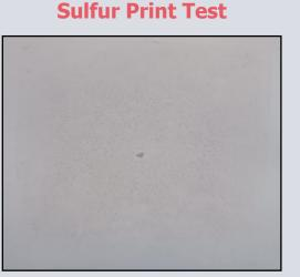
This test is used to check the distribution of sulfur in the sections of manufactured products with sulfur content between 0.01 and 0.40% by weight.
