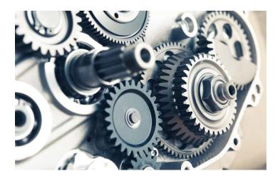
Gear materials are subjected to multiple load cycles during operation, and gear teeth experience high surface contact stresses, high bending stresses, typically in the root area, and potential sliding wear forces as the teeth move in and out of mesh. The contact stresses and bending stresses produce long-term fatigue damage.
