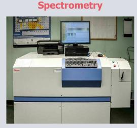
Spectrometry test is used to identify and measure the percentage of elements in products.
