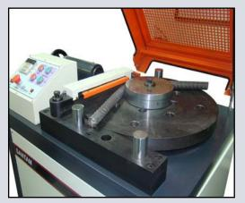
The bend and Rebend test are used to determine the quality of metals or welding against plastic deformation.
