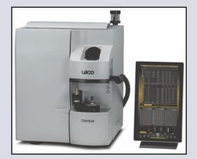
This test is to determine the amount of oxygen, nitrogen and hydrogen in the melting and casting process.
