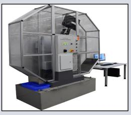
The Charpy impact test, is a standardized high strain rate test which determines the amount of energy absorbed by a material during fracture. Absorbed energy is a measure of the material's notch toughness. The parameters of absorbed energy, lateral expansion and percentage shear fracture are determined by this test.
